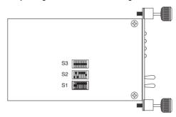
Figure 1. Location of DIP switches on Model 3088RC
